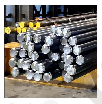
**080M50** is a type of medium carbon steel containing carbon, manganese, silicon, phosphorus, and sulphur.
