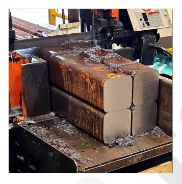
**080M46** steel is a high tensile strength steel with good machinability and wear resistance.
