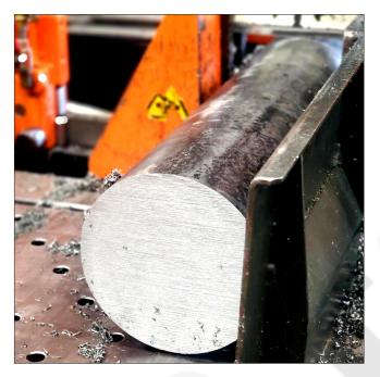
**070M20** (EN3A) is a low carbon, well-balanced unalloyed engineering steel suited where heavy stresses and heat treatment are not applied.
