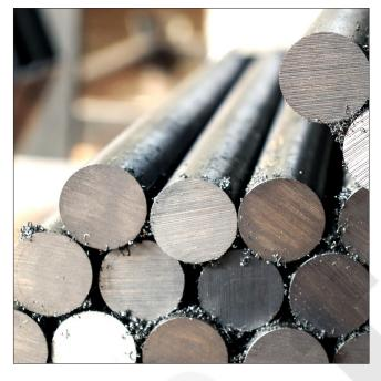
We stock **BO1 tool steel** which is oil-hardened containing chromium, vanadium & tungsten. The steel finds use in various applications, particularly in manufacturing much larger parts.
