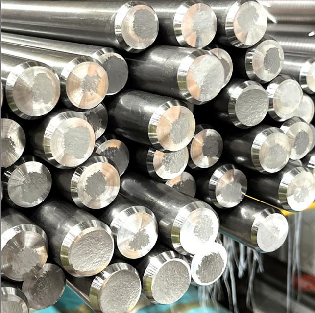
**605M36T (EN16T)** through-hardening low alloy engineering steel contains manganese and silicon.
