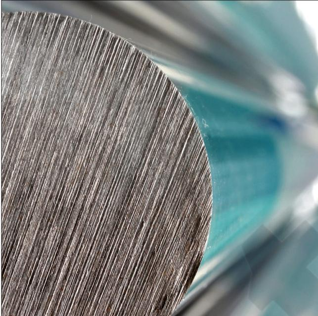
**27MnCrB5 (1.7182)** is a boron heat-treatable low alloy engineering steel that offers a cost-effective material solution compared to other steel grades.
