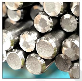
**709M40** is a type of high-tensile steel commonly used to construct engineering components, such as axles, gears, and shafts.
