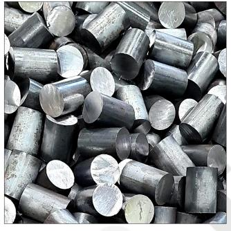
**708M40** is a high-tensile steel commonly used in applications that demand high strength and toughness, such as aerospace, automotive, and defence industries.
