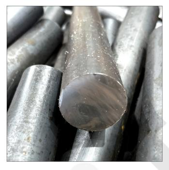
**42CrMo4** is a type of alloy steel that contains chromium and molybdenum as the main alloying elements.
